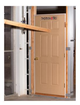
Built with a steel-plate inside to help withstand high-winds and damage from flying debris, Therma-Tru<sub>®</sub> Impact-rated door products are a better way to protect any home from weathergenerated hazards. We even shoot 8-foot long 2"x4" stud wood "missiles" at 35 mph into our doors to prove their strength and resistance to damage. When coupled with Impact-rated glass, our Impact-rated entryways create a complete package of beauty, style and protection.\*
